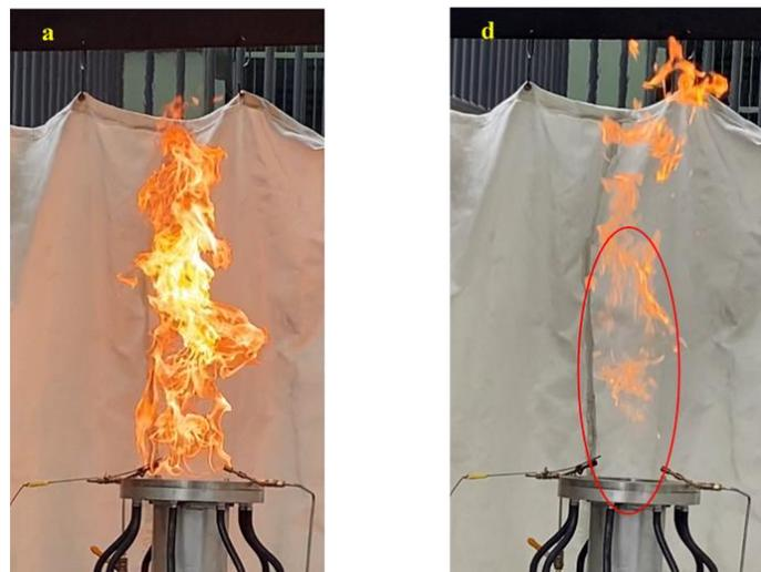
Figure 6 - Flame above Flare Tip with 20 L/min propane with: a) 0 cfm assist air, b) 12 cfm assist air
