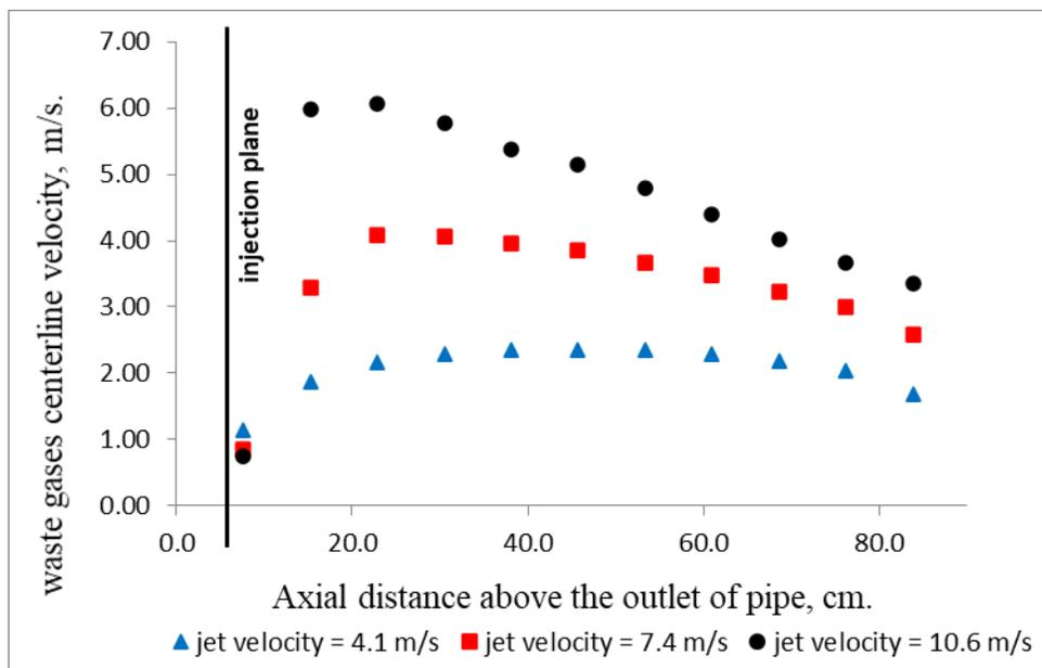
Figure 3 - Experimental measurements of flare gas centerline velocity for different slot jet flow
